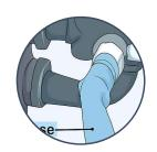
Make sure waste hose is securely connected to the valve
